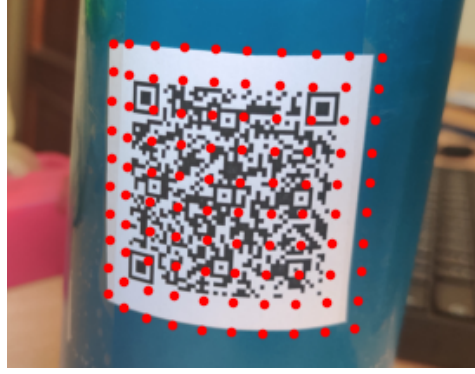
Figure 3.7: Example of sampling a transformation created with the cylindrical method
